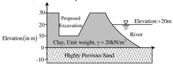
The water level in the adjacent river is at an elevation of +20.0m. Unit weight of water is 10kN/m<sup>3</sup>. The factor of safety (up to two decimal places) against sand boiling for the proposed excavation is
