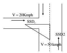
$$SSD_1 = v.t_r + \frac{v^2}{2g\mu} = \left(20 \times \frac{5}{18}\right) \times 2.5 + \frac{\left(20 \times \frac{5}{18}\right)^2}{2 \times 9.81 \times 0.38} = 13.89 + 4.139 = 18m$$
