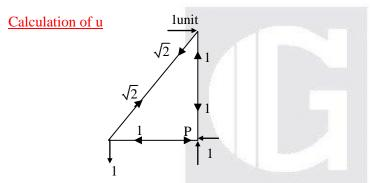
Applying 1 unit load in horizontal direction at C.
