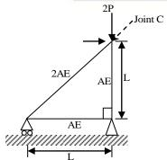
Given that  $E=2\times10^{11}$  N/m<sup>2</sup>, A=10mm<sup>2</sup>, L=1 m and P=1 kN. The horizontal displacement of joint C (in mm, up to one decimal place) is
