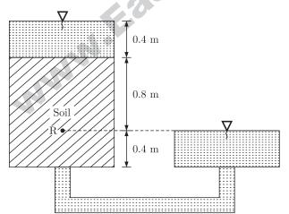
**Q. 46** The total head, elevation head and pressure head in metres of water at the point R shown in the figure are (A) 0.8 0.4 0.4 (B) 1.2 0.4 0.8
