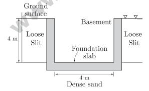
Using factor of safety = 3, the net safe bearing capacity (in  $kN/m^2$ ) of the foundation is:
