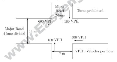
The critical lane volume on the major road changes to 440 vehicles per hour per lane and the critical lane volume on the minor road remains unchanged. The green time will
