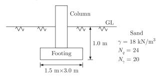
The net ultimate bearing capacity (kN/m²) of the footing based on Terzaghi's bearing capacity equation is
