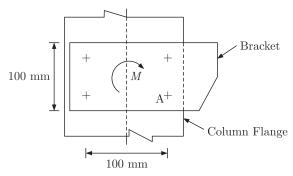
The shear force induced in the rivet A is
